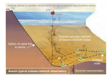
The same modularity concept is applied to the mechanical design. The usual deployment and maintenance procedures of the node imply the use of a submersible or a ROV, but free fall launching is possible. Among innovations : a low cost underwater connection system, a contact-less serial inductive link, an acoustic array mounted at the top of a flexible mast to have protection against trawlers.
