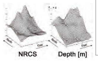
**Figure 1.** Grid map of he <u>N</u>ormalised <u>R</u>adar <u>C</u>ross <u>S</u>ection (NRCS) representing the small scaled sea surface roughness in comparison to the bathymetry of the test site "Lister deep".
