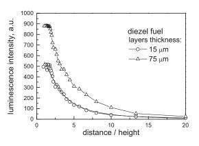
reliable detection may be provided by a low-cost, compact diode pumped solid state laser. Fluorescence signals in arbitrary units from different heights and for different distances are given in the figure above right. The graph shows that the inclination angle of laser beam excitation is the most limiting factor for scanning distance extension.
