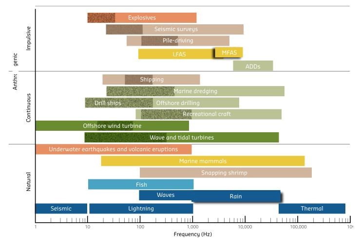
Figure 4. Comparing sound sources, where the order shows the relative sound pressure levels (dB) of the noise sources and the colour code allows comparison of the levels between categories (orange being highest dB level to dark blue being lowest). The areas with hatching indicate the frequency range with most energy. MFAS = Medium Frequency Active Sonar, LFAS = Low Frequency Active Sonar, ADD = Acoustic Deterrent Device
