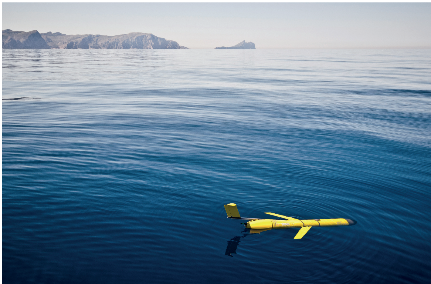
A Slocum Glider floats on the sea surface transmitting mission and sea state data via satellite to the IMEDEA (Mediterranean Institute for Advanced Studies) data facility.
