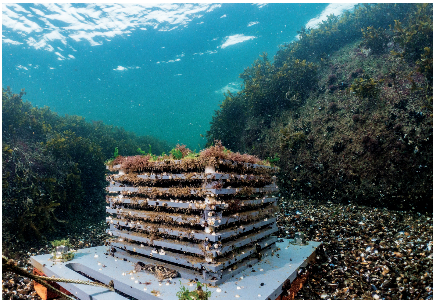
Artificial Reef Monitoring Structures (ARMS) function as biological forecasts for marine invasive species.
