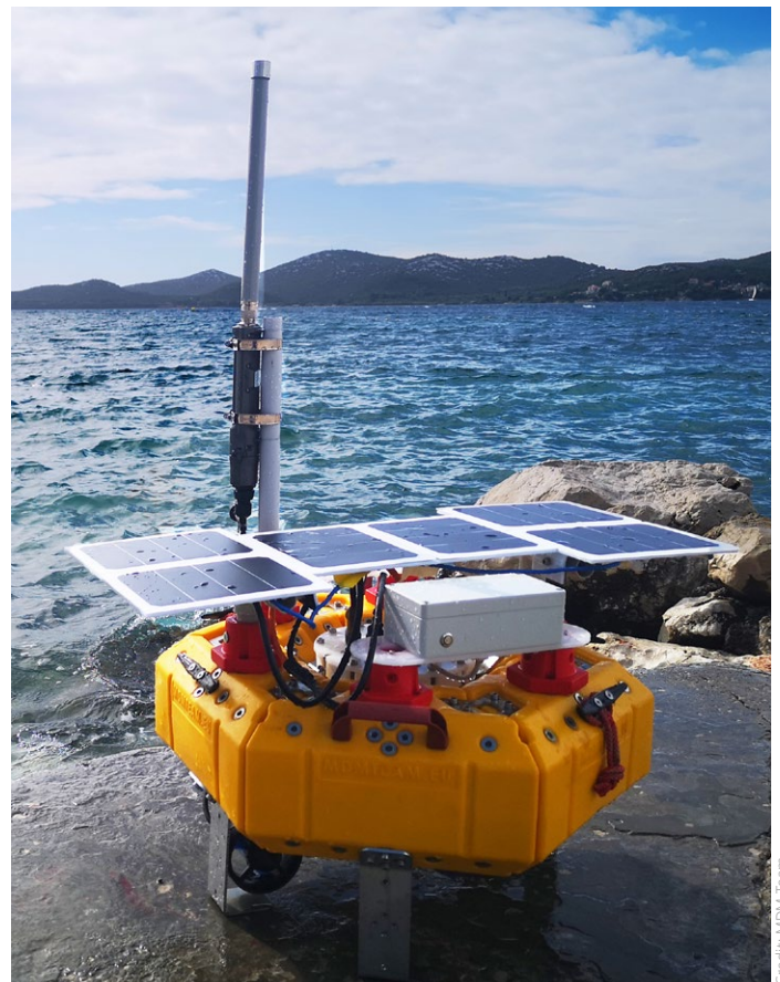
Figure 4: Monitoring node to collect water data during a trial.
