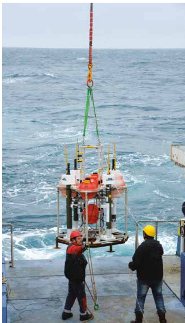
French Argo floats deployed during the 2017 Reykjanes Ridge Experiment (RREX) cruise (RV Atalante ) from an Autonomous System for Argo Float Research (ASFAR) structure.
