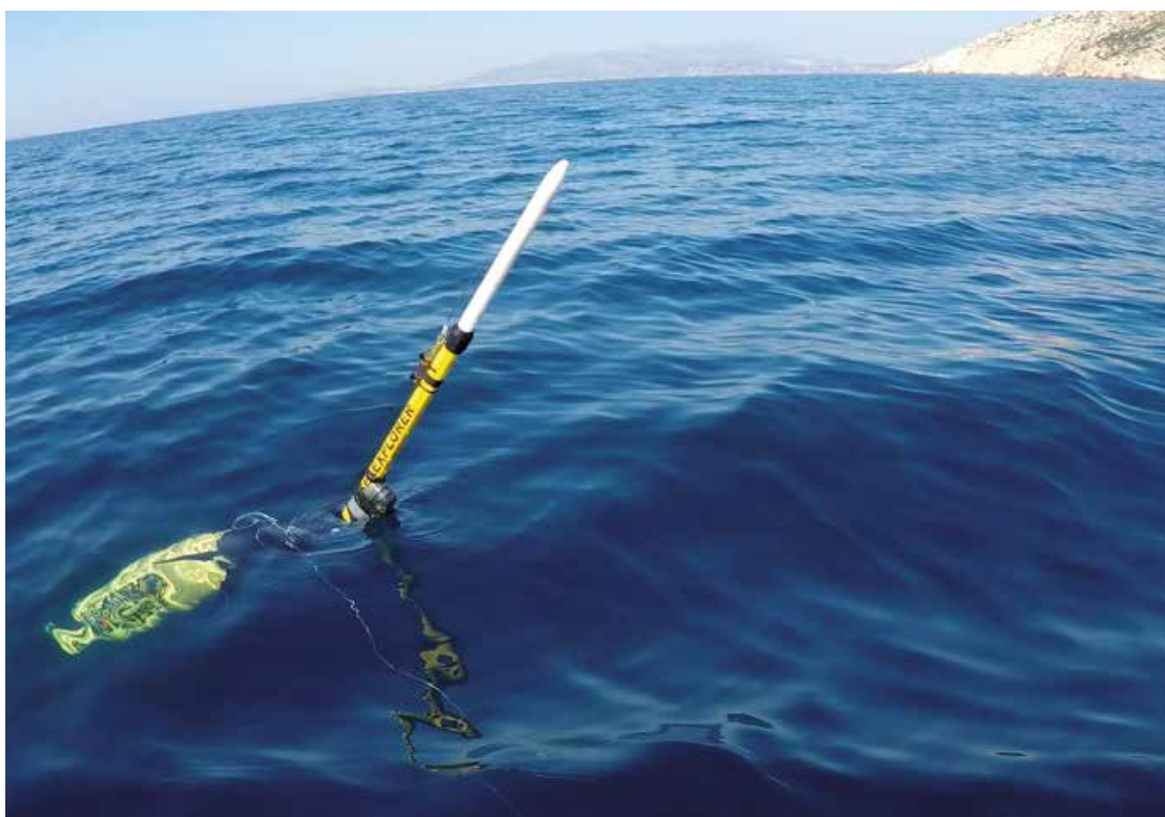
Monitoring cetaceans in the Cretan Sea using an acoustic receiver attached to a glider.
