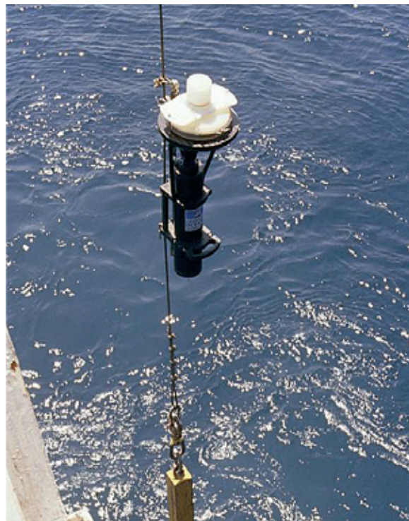
Figure 1.2. Sampling organic pollutants at sea with a high-volume sampling system
