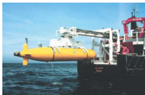
Recovery of AUTOSUB AUV from trials in Scottish sealoch using the RV Calanus . To date, AUTOSUB has achieved 240 autonomous missions with total track of 4600km without support ship control. © SOC Southampton, UK
