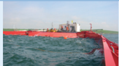
Figure 7: Wave Dragon - a floating, slack-moored energy converter off Nissum Bredning, Denmark
