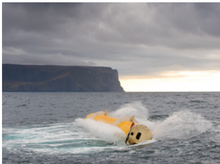
Figure 1: The first full-scale Oyster 1 wave power device in operation off Orkney coastline, Scotland
