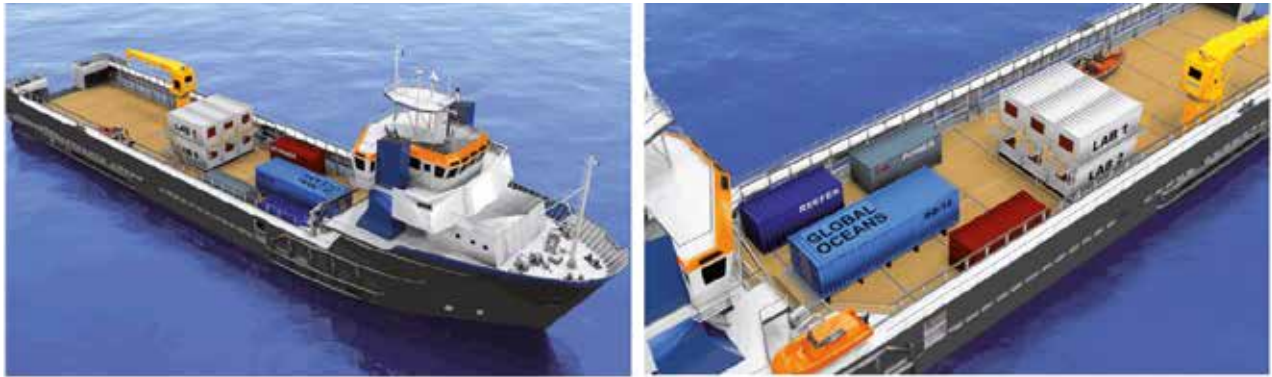
Fig. 6.12 Global Oceans science-configured OSV with modular laboratories, workshop, dry and cold storage, independent power supply, on-deck personnel housing, and operational support.
