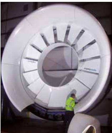
Fig. 3.20 Tidal turbine being prepared on land. The concept is being tested for use in the deep ocean.
