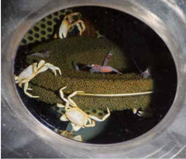
Fig. 6.13 AbyssBox. Live Segonzacia mesatlantica in the Abyss box maintained at 170bars.
