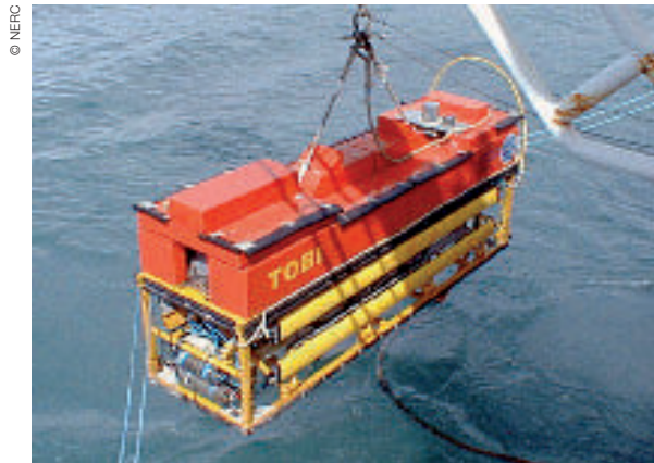
TOBI, a seafloor mapping system
