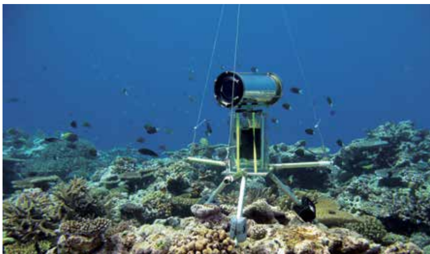
Remote underwater video system on a New Caledonian reef as part of a Marine Protected Area monitoring programme
