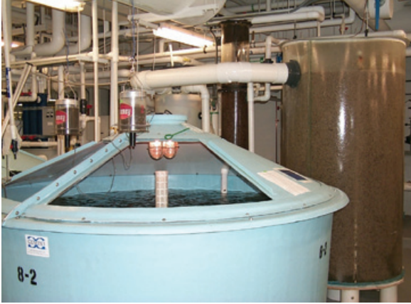
Figure 2.17. Recirculated fish tank with biofilter (drum on right), which uses beneficial microorganisms to remove chemical wastes from the water. (Courtesy Yonathan Zohar, COMB)
