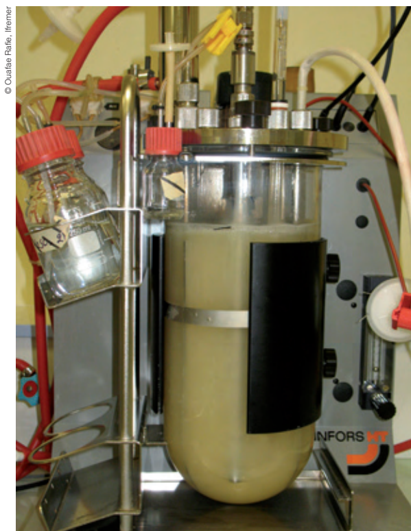
Figure 35. Experimental bioreactor for marine bacterial exopolysaccharide production
