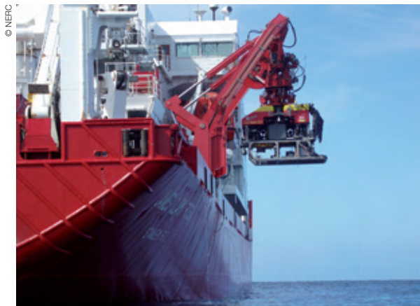
Figure 39. ROV deployment from RRS James Clark Ross operated by the National Oceanography Centre, Southampton, UK, on behalf of NERC.
