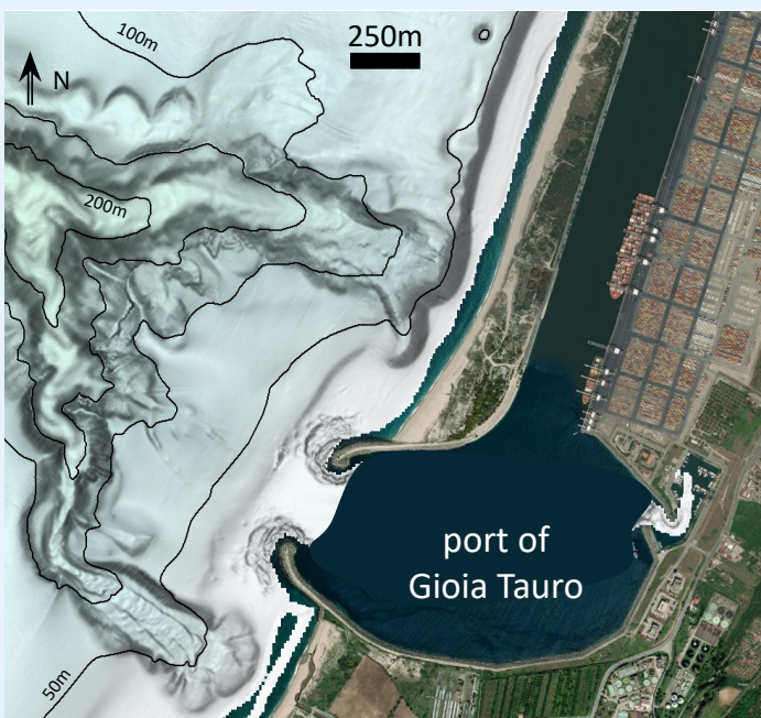
Figure 2.10. Multibeam bathymetry offshore Gioia Tauro port. Gioia Tauro is one of the main container ports of the Mediterranean and a possible entry point for emergency rescue vessels in case of a natural disaster in Calabria.
