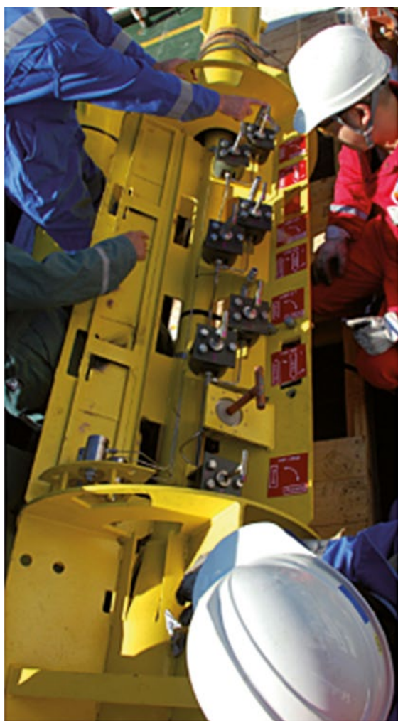
Figure 5.9. Left: One of the payload bays on the LTBMS head showing ROV-operable valves that allow fluid sampling as well as pump tests in the formation at up to several 100 meters sub-seafloor depth. Right: Head of an LTBMS surrounded by the ROV landing platform that also hosts a data recorder when it is lowered into the moonpool of DV Chikyu.
