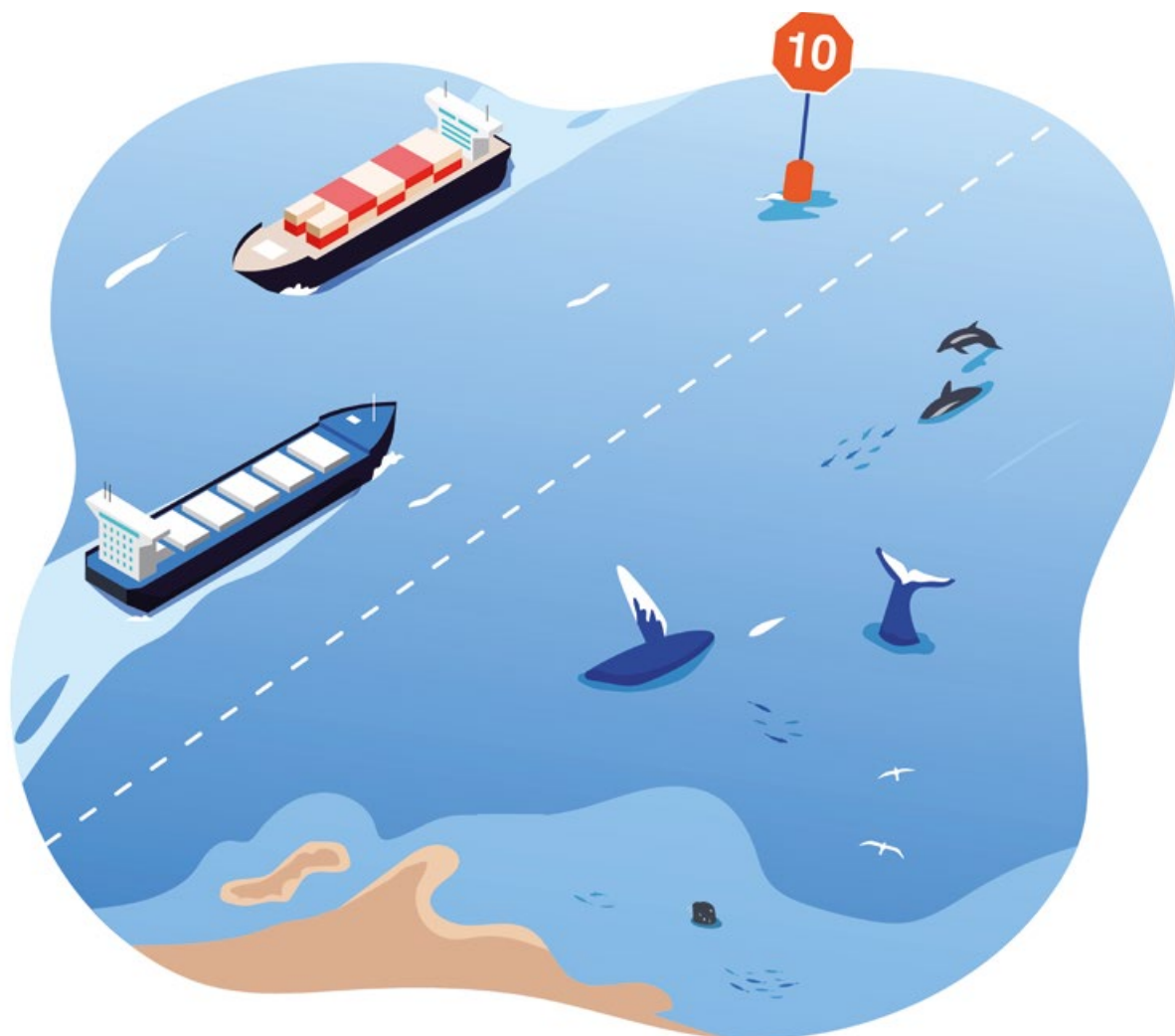
Figure 8. Traffic control strategies such as prescribed shipping routes and speed limits can be used in vulnerable areas.
