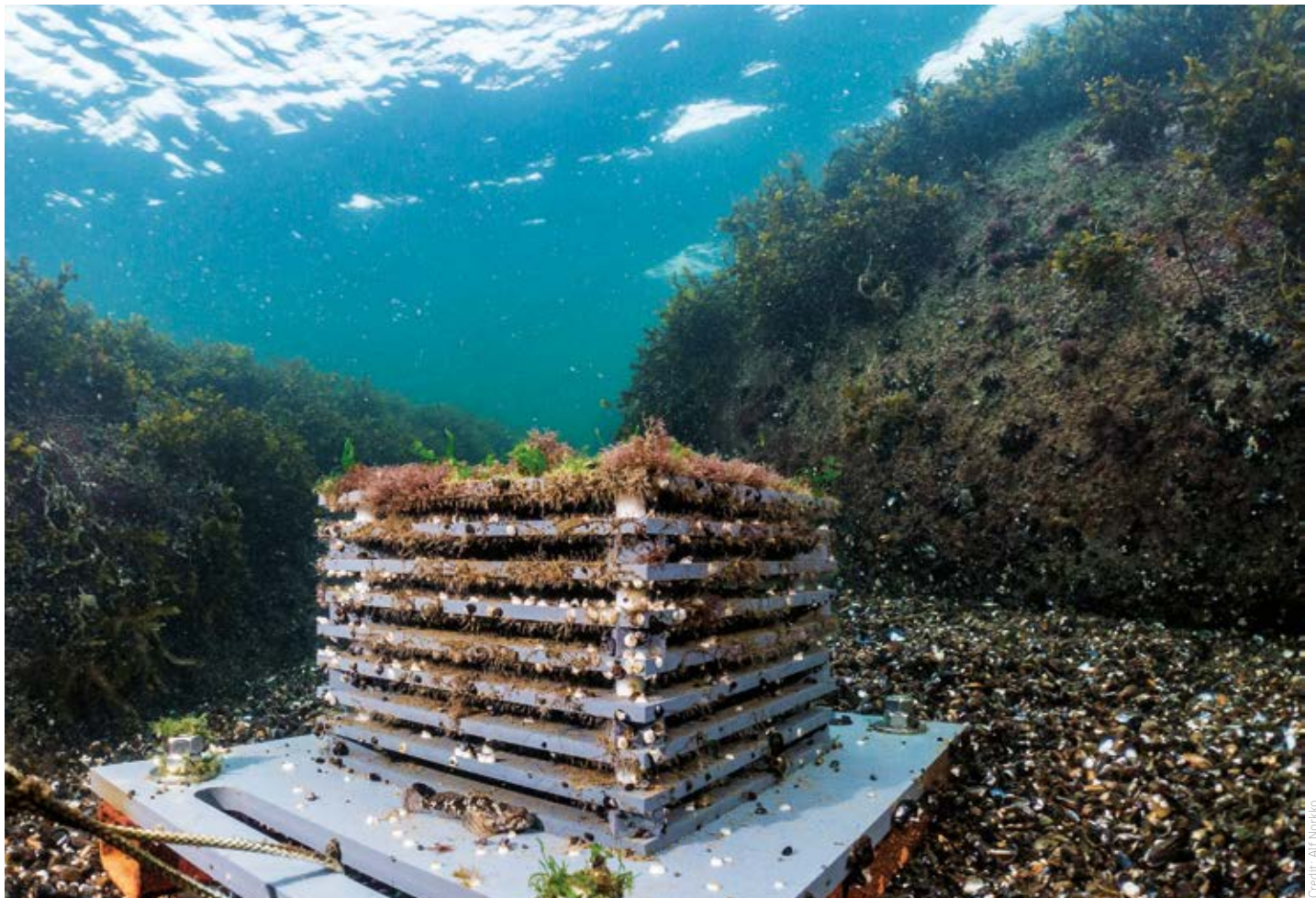
Artificial Reef Monitoring Structures (ARMS) function as biological forecasts for marine invasive species.
