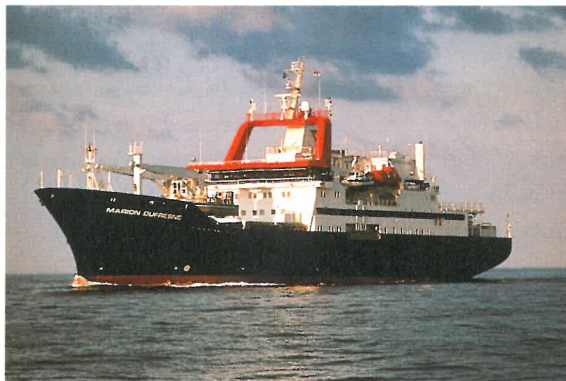
Fig. 5: R/V Marion Dufresne. She is a multipurpose vessel for logistics and oceanographic research. This vessel launched in 1995 is 120 metres long and 21 metres wide. She is operational in all oceanographic fields and, in particular, she is equipped with handling gear for high length core sampling of up to 60 metres. (Photo IFRTP, M. Le Coz)
