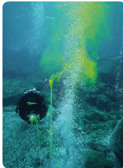
Use of dye to trace the water circulation around an underwater volcanic gas vent in Panarea Island, Southern Tyrrhenian Sea, Italy. Diver: R. Malatesta
